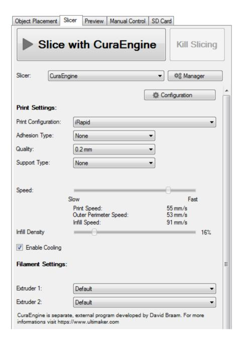
CuraEngine is external slicer software which is bundled with the Repetier-Host. Here you select your printing configurations to use plus some additional important settings. To define the parameters behind your configuration, click the "Configuration" button to enter the setup.
