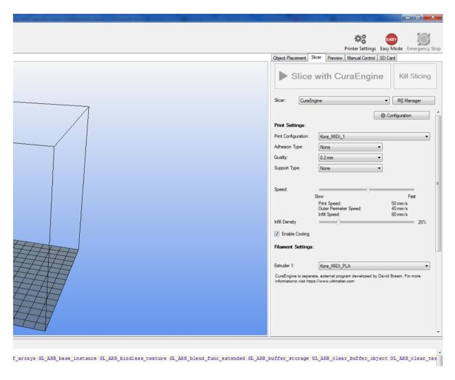
You can select any 'control option' in Repetier-Host, then hover your mouse over that setting and an 'explanation bubble' will appear guiding you how to use this option (eg. 'Adhesion Type', 'Support Type' etc etc.) This feature is particularly useful as it refers specifically to the control button or bar you have selected. Many controls throughout Repetier-Host have this feature! (see page 20 below for example)
