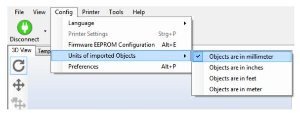
The Repetier-Host uses internally only millimetres. Unfortunately STL and OBJ format do not contain a scaling hint. Therefore you need to select the units used for the creation. That way the Repetier-Host will convert the units correctly into millimetres.
